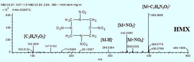
Figure 2. In-source CID TOF MS spectrum of HMX under DART negative mode by AccuTOF
