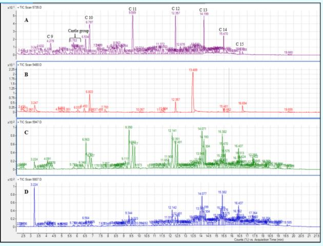
Figure 1: TICs for (A) 0.1% Kerosene reference, (B) Neat PE sample, (C) Burnt PE sample without kerosene and (D) Pyrolysed PE sample
