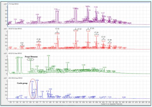
Figure 3: EIP for sample spiked with 15 µl kerosene
