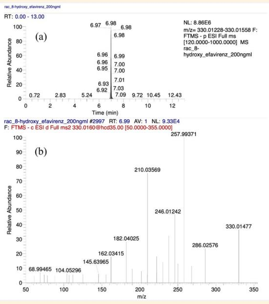
Figure 2. (a) Chromatogram and (b) ddMS2 spectrum of rac-8-bydroxy efavirenz at 200 ng/ml in LC-orbitrap-MS negative mode
