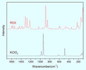
Figure 2: Raman spectra of RDX (above) and  $KCIO_3$  (below) particle
