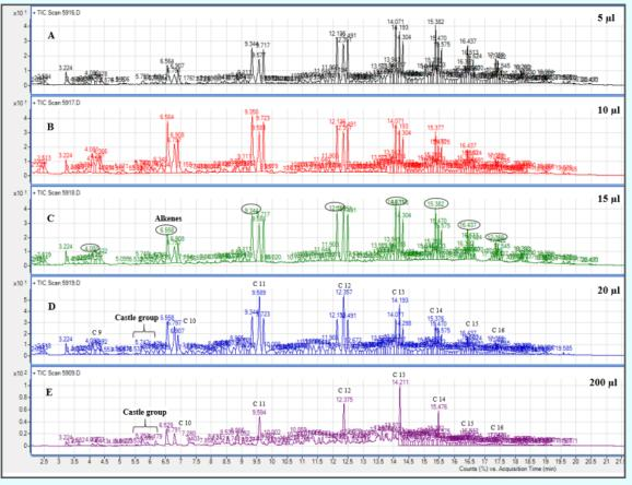
Figure 2: TICs for burnt PE samples spiked with kerosene of volume (A) 5  $\mu$ l, (B) 10  $\mu$ l, (C) 15  $\mu$ l, (D) 20  $\mu$ l and (E) 200  $\mu$ l
