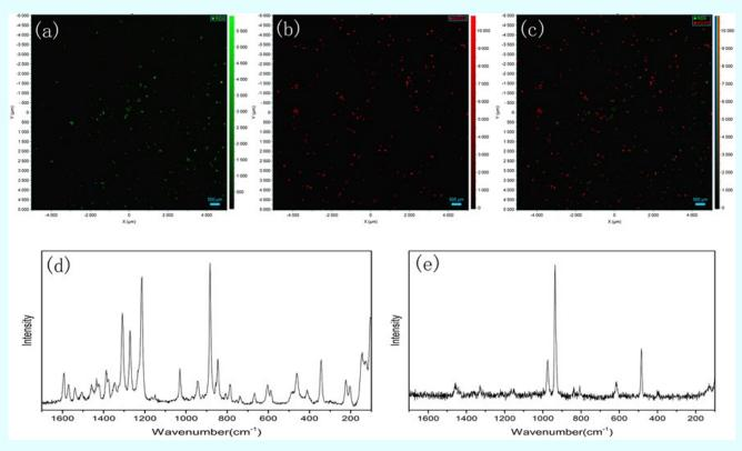
Figure 3: The distribution of explosive particles by selecting the characteristic Raman bands. (a) RDX distribution (870~900 cm<sup>-1</sup>); (b) KClO<sub>3</sub> distribution (470~500 cm<sup>-1</sup>); (c) RDX (green) and KClO<sub>3</sub> (red) distribution; (d) and (e) is the Raman spectra of RDX and KCIO3 particles on the sticky side of the tape respectively. (Spectral acquisition time: 500 ms; acquisition times: 1; laser power: 13.5 mW).
