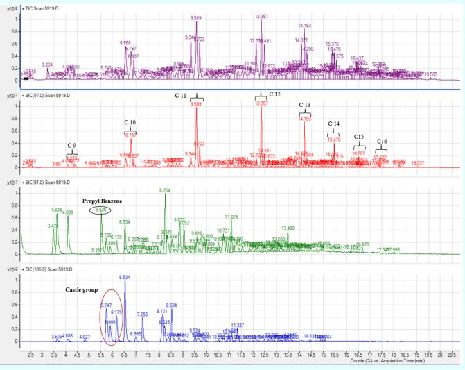
Figure 4: EIP for sample spiked with 20 µl kerosene
