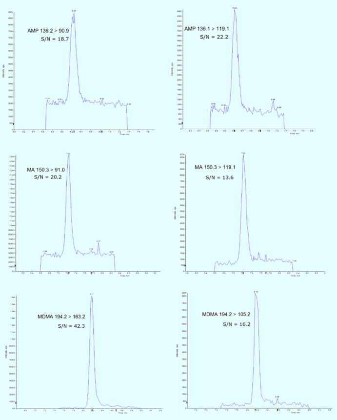
Figure 2. Chromatograms of AMP, MA and MDMA at 3 ng/mL
