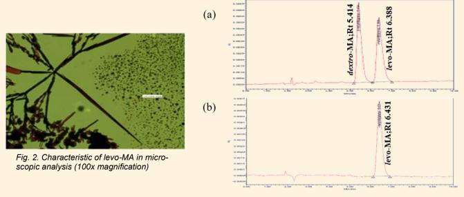
Fig. 3. Chirality analysis of (a) mixed of MA standards; (b) MA sample
