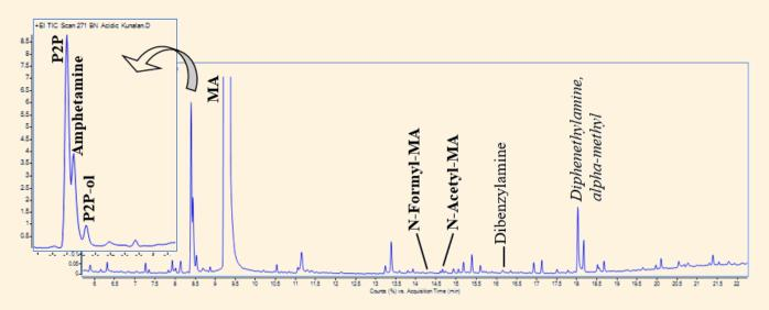
Fig. 4. Typical TIC of seized MA under acidic extraction
