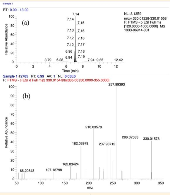
Figure 1. (a) Chromatogram and (b) ddMS<sup>2</sup> spectrum of a urine sample submitted for cannabinoids analysis.
