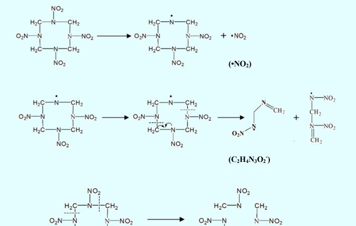
Figure 3. Proposed fragmentation pathway for the radical anions [M+ NO2]•- (m/z 342) and [M+ C2H4N3O2]•- (m/z 398) of HMX.
